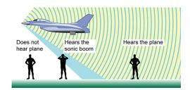
Figure 21.4: If a supersonic jet flew overhead, you would not hear the sound until the plane was far beyond you. The boundary between sound and silence is called a "shock wave." It is almost as if all the sound were compressed into a thin layer of air. The person in the middle hears a sonic boom as the shock wave passes over him. Because the sonic boom can shatter windows, planes are not allowed to fly over cities at supersonic speeds.
