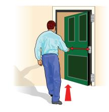
**Figure 5.22:** A door rotates around its hinges and a force creates the greatest torque when the force is applied far from the hinges.
