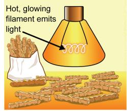
**Figure 22.2:** An incandescent light bulb generates light by heating a metal filament. The atoms inside the filament convert electrical energy to heat and then to light.
