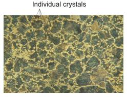
**Figure 8.7:** *Metallic crystals in steel. Single crystals are very small. This image is taken with an electron microscope at very high magnification.*
