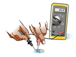
**Figure 13.12:** *A multimeter can be used to measure resistance of a device that has been completely removed from the circuit.*
