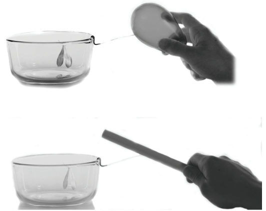
Bring different charged and uncharged objects near the wire.
