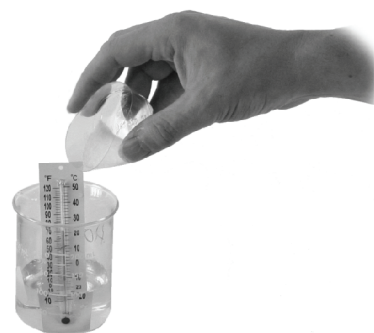
Add the calcium chloride to the water and stir gently with the thermometer
