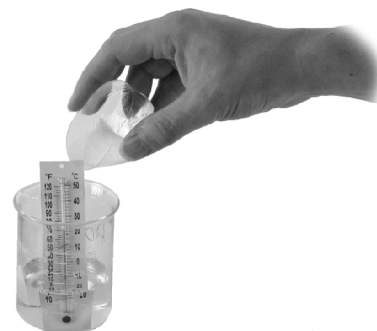
Add the ammonium nitrate to the water and stir gently with the thermometer.
