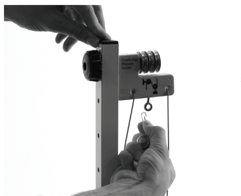
Connect string to the upper pulley block for mechanical advantage of 2,4, or 6.
